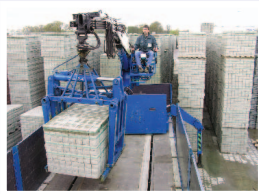
Brick and Block handling with Kennis clamp and pallet fork.
