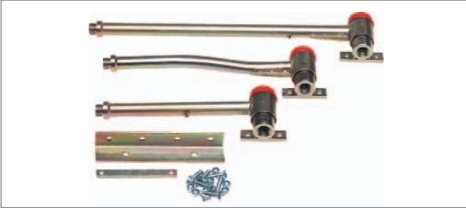
FLEX SAVER hose guide is a heavy duty design guide applicable for several possible tractor configurations. With several options of shapes and lengths can be applied in the most efficient way to keep the built height at minimum level. The arm rotates due to heavy duty swivel arm suitable for high pressure applications.
