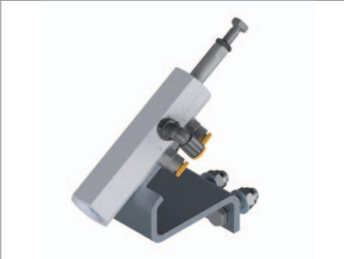
Knock off valve STD is mounted on the cylinder cradle, it is delivered with a special bracket to allow easy installation and precise setting of this limiter. It is pneumatically operated, the mechanical adjustment allows it to be used with full range of Hyva front cylinders. Usage of this valve assures precise operation and smooth limitation of the stroke which results in significant increase of the cylinder and hydraulic lit lifetime.
