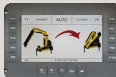
This easy-to-use function improves driver attention, promotes safety, saves time and increases productivity. Once the truck is stabilized, a graphic display allows the driver to automatically unfold the crane to a working position and fold the crane from any position to transport position.
