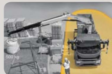
This system, a first on truck-mounted articulated cranes, optimises stabilization, makes crane operation safer and more efficient and allows the driver to verify in advance the crane lifting capacity based on truck stability.
